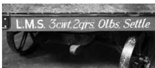
The trolley is of Midland Railway design of which there were, in all, 44 types (the LNWR had 34). The LMS categorised all the pre-grouping types into a total of 84 LMS standards. This is a MR Type 201, 9' 9" long over the wooden surface.
